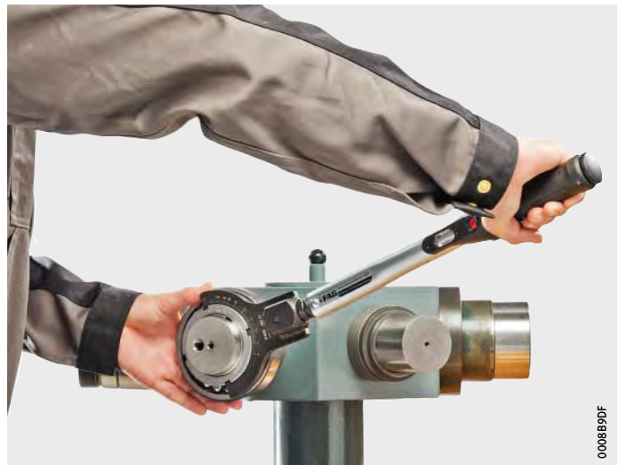
Figure 11 Mounting by means of double hook wrench
