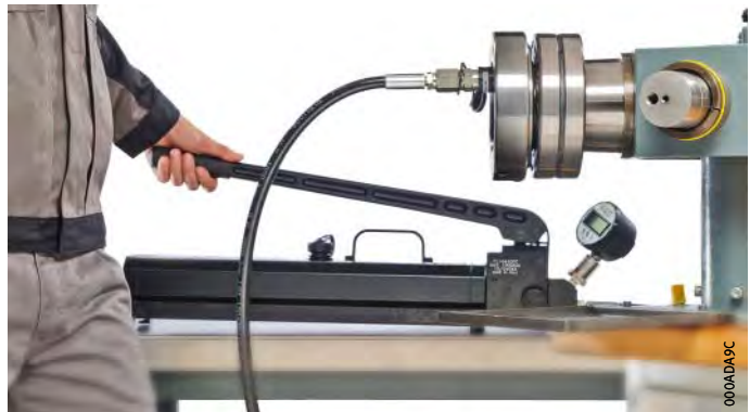
Figure 9 Hydraulic dismounting of tapered seat
