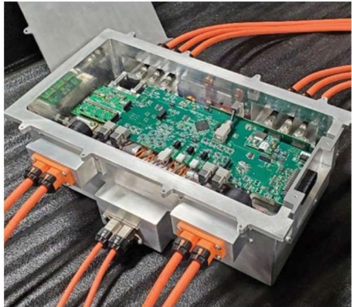
eLeap Power's integrated inverter takes advantage of the windings of an electric motor (when it's not moving) to replace a vehicle's onboard charger and its artificially slow charging speeds.
