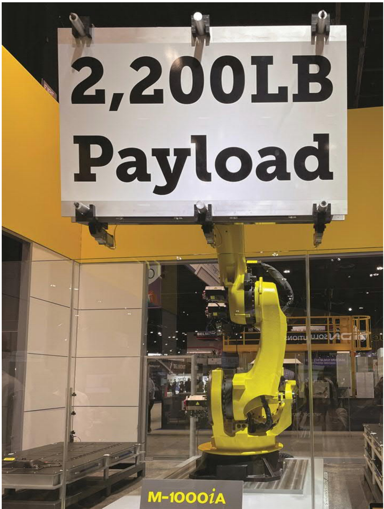
The FANUC M-1000iA robot, seen here handling a 1,000 kg EV battery pack in Booth 338919 at IMTS 2022
