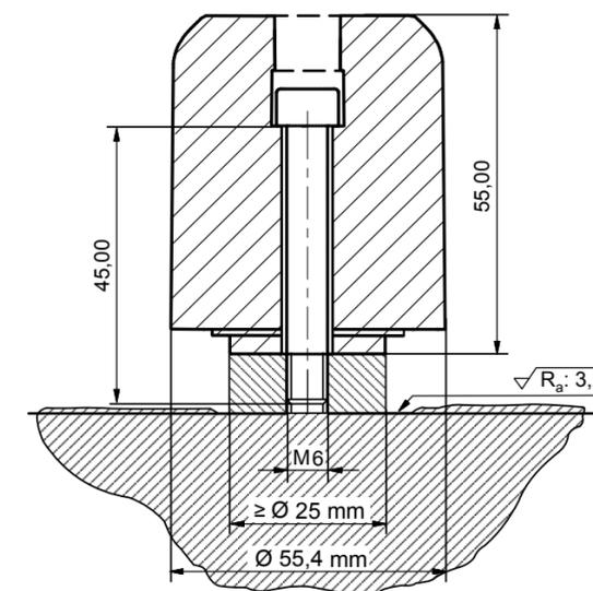
FAG SmartCheck installed with sensor mounting plate
