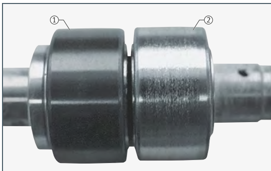
Figure 41 Comparison of coated and uncoated stud type track rollers
