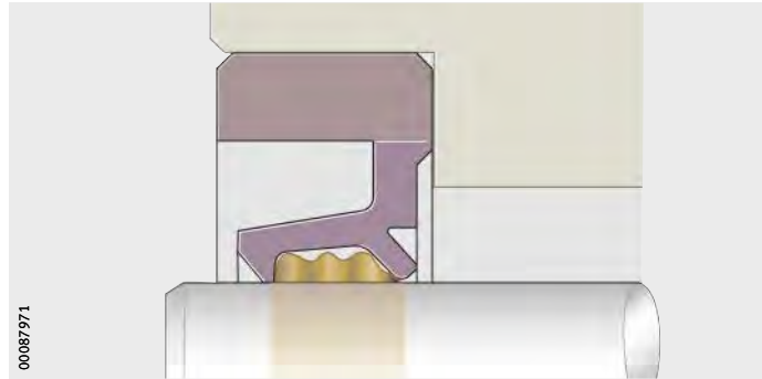
Figure 6 Grease filling between seal lip and protective lip
