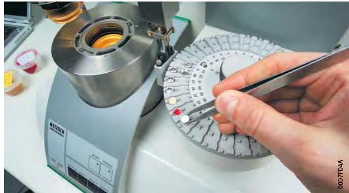
Figure 5 Analysis of the thermal behaviour of greases
