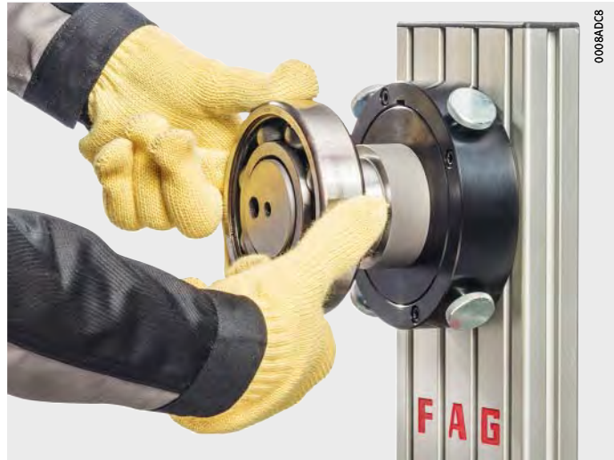
Figure 14 Sliding into place of heated bearing parts
