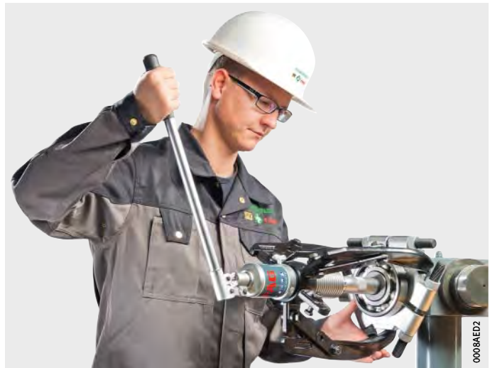
Figure 1 Dismounting by means of extraction device
