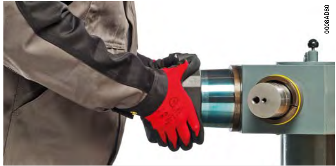
Figure 5 Touching with a taper ring gauge
