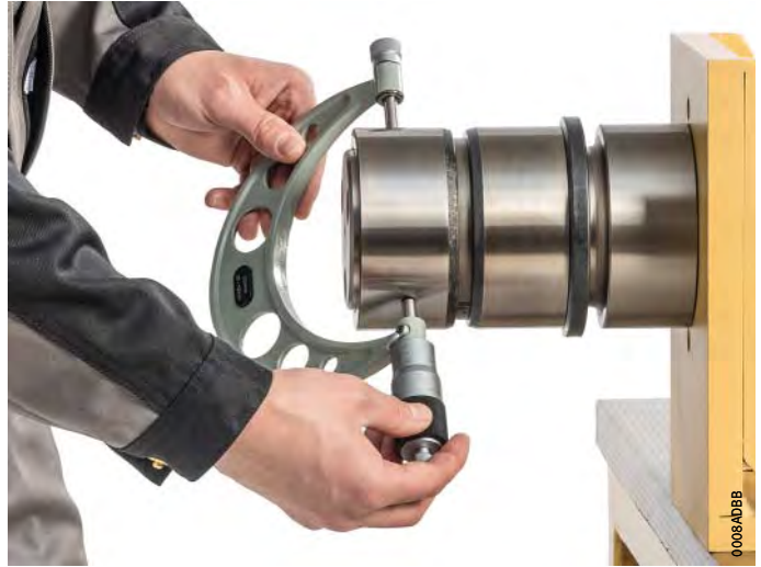
Figure 3 Measurement of expansion using external micrometer
