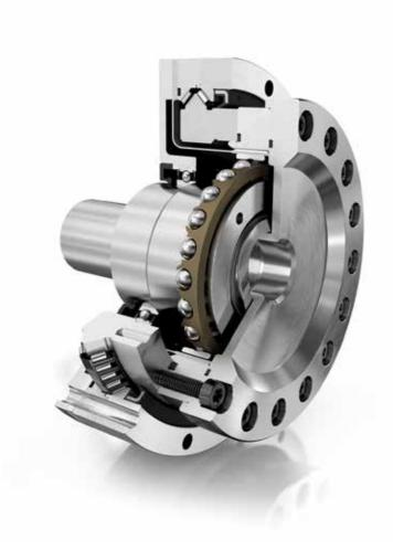
Schaeffler has used the highly rigid XZU angular contact needle roller bearings and flexsplines with optimized design and manufacturing processes to develop new strain wave gears, which have exceptionally high precision, torque density, and an outstandingly long operating life. The optimized 3D gear tooth geometry of the flexsplines allows a more even load distribution over the gearing and ensures complete tooth meshing. The precision gearing is also produced using forming
