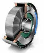
A new type of motor for robotics: Axial flux motor with coils in PCB design
