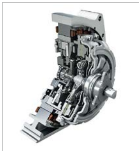
The Schaeffler hybrid module 48 Volt allows drive and recuperation.
